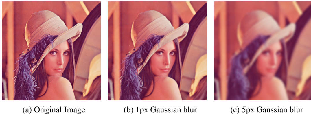
Figure 6.2: 512x512px “Lena”(a) with a 1px (b) and 5px (c) Gaussian blur applied. Gaussian blurring is accomplished by convolving an image with a Gaussian kernel and is commonly used in image processing to reduce noise prior to edge detection.
